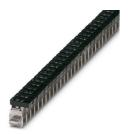
Connection terminal block, nom. voltage: 300 V, nominal current: 76 A, connection method: Screw connection, Rated cross section: 16 mm², cross section: 1.5 mm² - 16 mm², mounting: Neutral busbar, color: black
