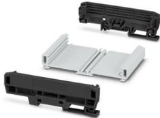
Profile housing (PA), mounting type: DIN rail mounting, dimensions on the DIN rail: width: 83.8 mm, height: 127.8 mm, depth: 39.45 mm, incl. 2 lateral elements (PA), color: black (9005), for PCBs with width: 108 mm, length: 80 mm, PCB surface: 6570 mm<sup>2</sup>
