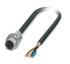
Device connector rear mounting, 4-position, PUR, black-gray RAL 7021, Socket, straight, M12-Push-Pull, coding: A, on free cable end, Rear mounting, M16 x 1.5, Individual wires, cable length: 2 m, PUR halogen-free black
