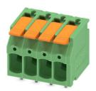
PCB terminal block, nominal current: 24 A, rated voltage (III/2): 400 V, nominal cross section: 2.5 mm<sup>2</sup>, number of potentials: 4, number of rows: 1, number of positions per row: 4, product range: LPT 2,5/, pitch: 5 mm, connection method: Lever Push-in connection, mounting: Wave soldering, conductor/PCB connection direction: 0 °, color: green, Pin layout: Linear pinning, Solder pin [P]: 3.5 mm, type of packaging: packed in cardboard
