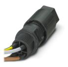
Panel feed-through, product family: QPD, connection method: Single wires (Welded-on)/ IDC connection, number of positions: 3+PE, M25, Pin, 1 mm<sup>2</sup> ... 2.5 mm<sup>2</sup>, 690 V, 20 A, PA, black, with QUICKON nut, external cable diameter: 9 mm ... 14 mm, 2.5 mm<sup>2</sup>, wires cut flat at the end, cable length: 0.5 m, with additional SEALING PLUG 14X22 RD
