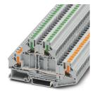
Double-level terminal block, nom. voltage: 1000 V, nominal current: 28 A, connection method: Push-in connection, 1st and 2nd level, Rated cross section:  $4 \text{ mm}^2$ , cross section:  $0.2 \text{ mm}^2$  -  $6 \text{ mm}^2$ , color: gray
