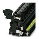
Fuse modular terminal block, fuse type: Glass / ceramics / ..., fuse type: G / 5 x 20, nom. voltage: 250 V, nominal current: 6.3 A, connection method: Screw connection, Rated cross section: 1  $mm^2$ , cross section: 0.14  $mm^2$ - 6  $mm^2$ , mounting type: NS 35/7,5, NS 35/15, color: black
