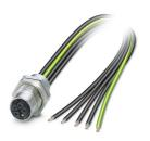
Device connector rear mounting, Power, 5-position, Socket, straight, M12-Standard, coding: K, on free cable end, Rear mounting, M16 x 1.5, Individual wires, cable length: 1 m, 1.31 mm<sup>2</sup>, UL/cUL stranded hook-up wire, Alternative product in accordance with RoHS II without Exemption 6c (Pb < 0.1 %) item no.: 1238589
