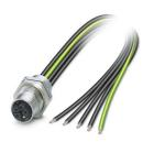
Device connector rear mounting, Power, 5-position, Socket, M12, coding: K, on free cable end, Rear mounting, M16 x 1.5, Individual wires, cable length: 1.5 m, 2.50 mm<sup>2</sup>, PEX litz wire, Alternative product in accordance with RoHS II without Exemption 6c (Pb < 0.1 %) item no.: 1238541
