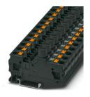
Fuse modular terminal block, fuse type: Glass / ceramics / ..., fuse type: G / 5 x 20, nom. voltage: 24 V, nominal current: 10 A, connection method: Push-in connection, Rated cross section: 6 mm<sup>2</sup>, cross section: 0.5 mm<sup>2</sup>- 10 mm<sup>2</sup>, mounting type: NS 35/7,5, NS 35/15, color: black
