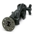
140.5 mm housing attachment, for max. load 10 kg, with ball joint and fastening plate 60 mm, pivotable in 15° increments, for 30 mm wall/profile bracket, material: black glass-fiber reinforced polycarbonate PC, and black anodized aluminum, 342 g
