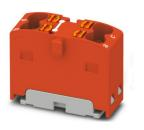
Distribution block, bridged internally, nom. voltage: 450 V, nominal current: 17.5 A, number of connections: 4, connection method: Push-in connection, cross section: 0.14 mm<sup>2</sup> - 2.5 mm<sup>2</sup>, mounting type: for snapping onto a DIN rail adapter, Direct mounting with flange, Free-hanging, color: red
