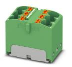
Distribution block, bridged internally, nom. voltage: 450 V, nominal current: 32 A, number of connections: 6, connection method: Push-in connection, cross section:  $0.2 \text{ mm}^2$  - 6 mm<sup>2</sup>, mounting type: adhesive, color: green
