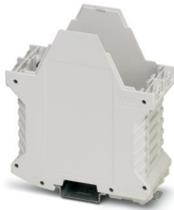
DIN rail housing, Lower housing part with metal foot catch, with FE contact, tall design, with vents, width: 45.2 mm, height: 99 mm, depth: 107.3 mm, color: light grey (similar RAL 7035), cross connection: DIN rail connector (optional), number of positions cross connector: 5
