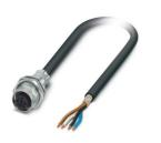
Device connector rear mounting, 4-position, PUR, black-gray RAL 7021, Socket, straight, M12-SPEEDCON, coding: A, on free cable end, Rear mounting, M16 x 1.5, Cable connection, cable length: 3 m, 0.34 mm<sup>2</sup>, PUR halogen-free black, Alternative product in accordance with RoHS II without Exemption 6c (Pb < 0.1 %) item no.: 1238286
