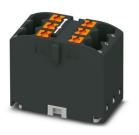
Distribution block, Basic terminal block, nom. voltage: 450 V, nominal current: 24 A, number of connections: 6, connection method: Push-in connection, cross section: 0.14 mm<sup>2</sup> - 4 mm<sup>2</sup>, mounting type: adhesive, color: black
