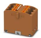
Distribution block, Basic terminal block, nom. voltage: 450 V, nominal current: 24 A, number of connections: 6, connection method: Push-in connection, cross section: 0.14  $\text{mm}^2$  - 4  $\text{mm}^2$ , mounting type: adhesive, color: brown
