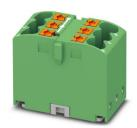
Distribution block, Basic terminal block, nom. voltage: 450 V, nominal current: 24 A, number of connections: 6, connection method: Push-in connection, cross section: 0.14  $\text{mm}^2$  - 4  $\text{mm}^2$ , mounting type: adhesive, color: green
