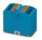
Distribution block, Basic terminal block, nom. voltage: 450 V, nominal current: 24 A, number of connections: 6, connection method: Push-in connection, cross section: 0.14 mm<sup>2</sup> - 4 mm<sup>2</sup>, mounting type: adhesive, color: blue
