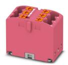
Distribution block, Basic terminal block, nom. voltage: 450 V, nominal current: 24 A, number of connections: 6, connection method: Push-in connection, cross section: 0.14 mm² - 4 mm², mounting type: for snapping onto a DIN rail adapter, Direct mounting with flange, Free-hanging, color: pink
