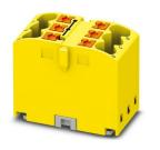
Distribution block, Basic terminal block, nom. voltage: 450 V, nominal current: 24 A, number of connections: 6, connection method: Push-in connection, cross section: 0.14 mm<sup>2</sup> - 4 mm<sup>2</sup>, mounting type: for snapping onto a DIN rail adapter, Direct mounting with flange, Free-hanging, color: yellow
