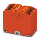
Distribution block, Basic terminal block, nom. voltage: 450 V, nominal current: 24 A, number of connections: 6, connection method: Push-in connection, cross section: 0.14 mm<sup>2</sup> - 4 mm<sup>2</sup>, mounting type: for snapping onto a DIN rail adapter, Direct mounting with flange, Free-hanging, color: red
