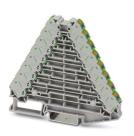
Marshalling panel, nom. voltage: 250 V, nominal current: 8 A, connection method: Push-in connection, 1st, 2nd, 3rd, 4th, 5th, 6th, 7th and 8th level, Rated cross section: 1.5 mm<sup>2</sup>, cross section: 0.14 mm<sup>2</sup> - 2.5 mm<sup>2</sup>, mounting: NS 35/7,5, NS 35/15, color: gray, color of connection elements: green
