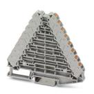
Marshalling panel, nom. voltage: 250 V, nominal current: 8 A, connection method: Push-in connection, 1st, 2nd, 3rd, 4th, 5th, 6th, 7th and 8th level, Rated cross section: 1.5 mm<sup>2</sup>, cross section: 0.14 mm<sup>2</sup> - 2.5 mm<sup>2</sup>, mounting: NS 35/7,5, NS 35/15, color: gray, color of connection elements: gray
