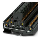
Fuse modular terminal block, fuse type: Glass / ceramics / ..., fuse type: G / 5 x 20, nom. voltage: 500 V, nominal current: 28 A, connection method: Push-in connection, 1 level, Rated cross section: 4 mm $^2$ , cross section: 0.2 mm $^2$ - 6 mm $^2$ , connection method: Push-in connection, 2nd level, Rated cross section: 4 mm $^2$ , cross section: 0.2 mm $^2$ - 6 mm $^2$ , mounting type: NS 35/7,5, NS 35/15, color: black
