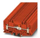
Disconnect terminal block, nom. voltage: 1000 V, nominal current: 41 A, connection method: Screw connection, 1 level, Rated cross section:  $6~\text{mm}^2$ , cross section:  $0.2~\text{mm}^2$  -  $10~\text{mm}^2$ , mounting type: NS 35/7,5, NS 35/15, NS 32, color: red
