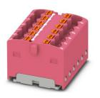
Distribution block, bridged internally, nom. voltage: 450 V, nominal current: 17.5 A, number of connections: 12, connection method: Push-in connection, cross section: 0.14 mm<sup>2</sup> - 2.5 mm<sup>2</sup>, mounting type: adhesive, color: pink
