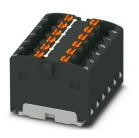
Distribution block, bridged internally, nom. voltage: 450 V, nominal current: 17.5 A, number of connections: 12, connection method: Push-in connection, cross section: 0.14 mm<sup>2</sup> - 2.5 mm<sup>2</sup>, mounting type: adhesive, color: black
