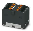
Distribution block, bridged internally, nom. voltage: 450 V, nominal current: 17.5 A, number of connections: 6, connection method: Push-in connection, cross section: 0.14 mm<sup>2</sup> - 2.5 mm<sup>2</sup>, mounting type: adhesive, color: black
