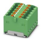
Distribution block, bridged internally, nom. voltage: 450 V, nominal current: 17.5 A, number of connections: 12, connection method: Push-in connection, cross section:  $0.14~\text{mm}^2$  -  $2.5~\text{mm}^2$ , mounting type: adhesive, color: green
