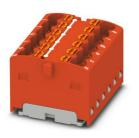
Distribution block, bridged internally, nom. voltage: 450 V, nominal current: 17.5 A, number of connections: 12, connection method: Push-in connection, cross section: 0.14 mm<sup>2</sup> - 2.5 mm<sup>2</sup>, mounting type: adhesive, color: red
