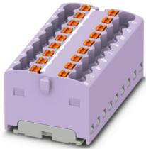
Distribution block, bridged internally, nom. voltage: 450 V, nominal current: 17.5 A, number of connections: 18, connection method: Push-in connection, cross section: 0.14 mm<sup>2</sup> - 2.5 mm<sup>2</sup>, mounting type: for snapping onto a DIN rail adapter, Direct mounting with flange, Free-hanging, color: violet
