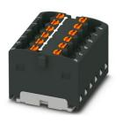
Distribution block, bridged internally, nom. voltage: 450 V, nominal current: 17.5 A, number of connections: 12, connection method: Push-in connection, cross section: 0.14 mm<sup>2</sup> - 2.5 mm<sup>2</sup>, mounting type: for snapping onto a DIN rail adapter, Direct mounting with flange, Free-hanging, color: black
