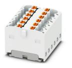
Distribution block, bridged internally, nom. voltage: 450 V, nominal current: 17.5 A, number of connections: 12, connection method: Push-in connection, cross section:  $0.14 \text{ mm}^2 - 2.5 \text{ mm}^2$ , mounting type: for snapping onto a DIN rail adapter, Direct mounting with flange, Free-hanging, color: white
