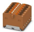
Distribution block, bridged internally, nom. voltage: 450 V, nominal current: 17.5 A, number of connections: 12, connection method: Push-in connection, cross section: 0.14 mm<sup>2</sup> - 2.5 mm<sup>2</sup>, mounting type: for snapping onto a DIN rail adapter, Direct mounting with flange, Free-hanging, color: brown
