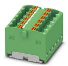
Distribution block, bridged internally, nom. voltage: 450 V, nominal current: 17.5 A, number of connections: 12, connection method: Push-in connection, cross section:  $0.14~\text{mm}^2$  -  $2.5~\text{mm}^2$ , mounting type: for snapping onto a DIN rail adapter, Direct mounting with flange, Free-hanging, color: green
