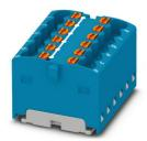
Distribution block, bridged internally, nom. voltage: 450 V, nominal current: 17.5 A, number of connections: 12, connection method: Push-in connection, cross section: 0.14 mm<sup>2</sup> - 2.5 mm<sup>2</sup>, mounting type: for snapping onto a DIN rail adapter, Direct mounting with flange, Free-hanging, color: blue
