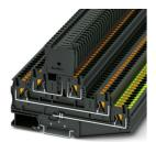
Fuse modular terminal block, fuse type: Glass / ceramics / ..., fuse type: G /  $5 \times 20$ , nom. voltage: 500 V, nominal current: 28 A, connection method: Push-in connection, Rated cross section: 4 mm², cross section: 0.2 mm²-  $6 \text{ mm}^2$ , connection method: Push-in connection, cross section: 0.2 mm²-  $6 \text{ mm}^2$ , mounting type: NS 35/7,5, NS 35/15, color: black
