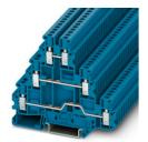
Multi-level terminal block, nom. voltage: 500 V, nominal current: 19 A, connection method: Screw connection, Rated cross section:  $2.5 \text{ mm}^2$ , cross section:  $0.14 \text{ mm}^2$  -  $4 \text{ mm}^2$ , mounting type: NS 35/7.5, NS 35/15, color: blue
