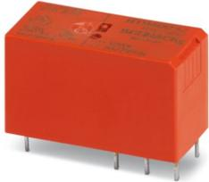
Plug-in miniature power relay, RT III sealed with power contacts, 2 changeover contacts, input voltage: 12 V DC, in connection with the corresponding PLC base approved in accordance with ATEX/IECEx (zone 2) and Ex zone class I, div. 2.
