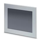
Touch panel with 38.1 cm/15" TFT-display (analog resistive (polyester)), 1024 x 768 pixel(s) (XGA), 65536 colors, Arm® Cortex®-A8, 800 MHz, 2x USB host 2.0, 1 x Ethernet (10/100 Mbps), RJ45, Windows® Embedded Compact 7 and user software: Visu+ / AX OPC Server. (bus system: without)
