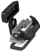
Panel mounting base D25, with single locking latch, material: Die-cast aluminum, salt water resistant, protective cover material: PC, height: 26 mm, cable gland: none, protective cover: yes, Standard
