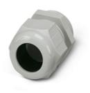
Cable gland, material for screw connection: PA, external cable diameter 19 mm ... 28 mm, shielding: no, connecting thread: M40 x 1.5, color: lightgrey RAL 7035
