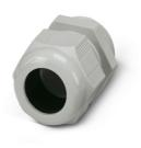
Cable gland, material for screw connection: PA, external cable diameter 15 mm ... 21 mm, shielding: no, connecting thread: M32 x 1.5, color: lightgrey RAL 7035
