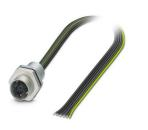
Device connector front mounting, Power, 6-position, Socket, straight, M12-Standard, coding: M, on free cable end, Front mounting, M16 x 1.5, Individual wires, cable length: 0.2 m, 1.31 mm<sup>2</sup>, UL/cUL stranded hook-up wire, Alternative product in accordance with RoHS II without Exemption 6c (Pb < 0.1 %) item no.: 1239087
