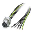
Device connector rear mounting, Power, 5-position, Socket, straight, M12-Standard, coding: K, on free cable end, Rear mounting, M16 x 1.5, Individual wires, cable length: 0.2 m, 2.50 mm<sup>2</sup>, PEX litz wire, Alternative product in accordance with RoHS II without Exemption 6c (Pb < 0.1 %) item no.: 1239081
