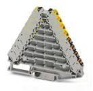
Potential distributors, nom. voltage: 250 V, nominal current: 17.5 A, connection method: Push-in connection, 1st, 2nd, 3rd, 4th, 5th, 6th, 7th and 8th level, Rated cross section: 1.5 mm², cross section: 0.14 mm² - 2.5 mm², mounting: NS 35/7,5, NS 35/15, color: gray, color of connection elements: yellow, black
