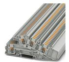
Installation level terminal block, nom. voltage: 400 V, nominal current: 28 A, Push-in connection, 1st, 2nd and 3rd level, Rated cross section: 4 mm², cross section: 0.2 mm² - 6 mm², Push-in connection, mounting type: NS 35/7,5, NS 35/15, color: gray
