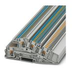
Installation level terminal block, nom. voltage: 400 V, nominal current: 28 A, Push-in connection, 1st, 2nd and 3rd level, Rated cross section: 4 mm<sup>2</sup>, cross section: 0.2 mm<sup>2</sup> - 6 mm<sup>2</sup>, Push-in connection, mounting type: NS 35/7,5, NS 35/15, color: gray
