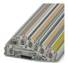
Installation ground terminal block, nom. voltage: 400 V, nominal current: 28 A, Push-in connection, 1st, 2nd and 3rd level, Rated cross section: 4 mm², cross section: 0.2 mm² - 6 mm², Push-in connection, mounting type: NS 35/7,5, NS 35/15, color: gray
